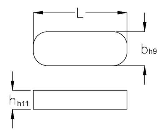
b = 12 h = 8 L = 30.0Tolerance b = 0.043Tolerance h = 0.090
